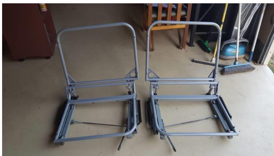
The two front seat frames, repaired and freshly powder-coated. The runners have been freed up and now work like a charm.
