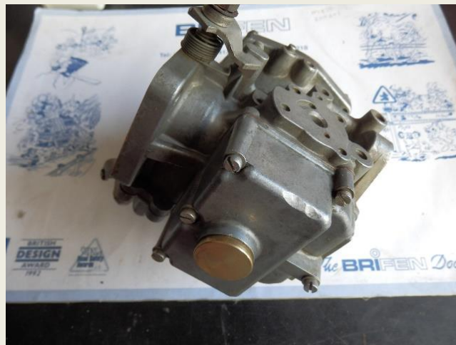
Base of Float Chamber Fretted by Steel Braided Petrol Return Pipe
