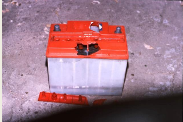
Original Jaguar V12 'E' Type Lucas "Pacemaker" Battery Shattered after Explosion
